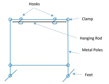
\*Clamps require a 13mm spanner or socket or shifter
