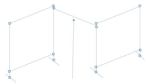
Two freestanding fames can be linked using a metal pole as Joiner – only one required at top
